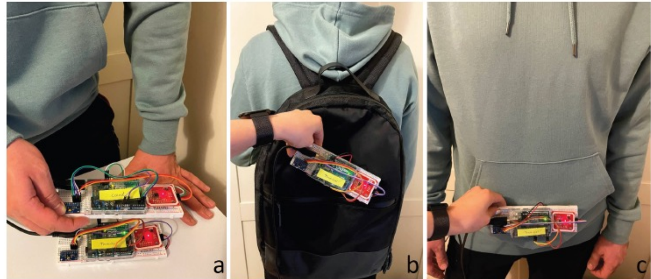
a) OPay payment setup; b) random guessing attack; c) targeted guessing attack
