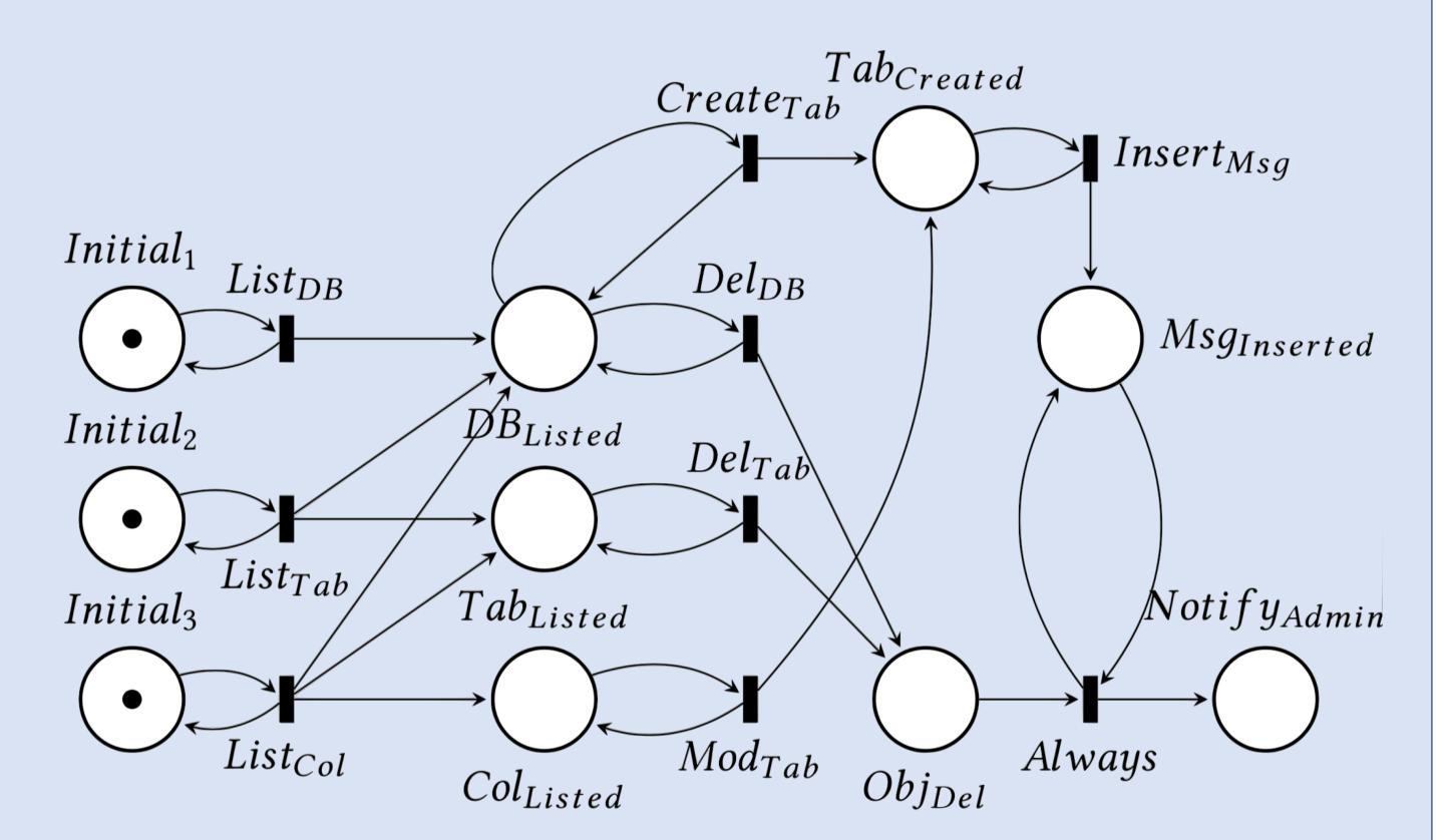
Representation of the CPN used to detect current ransomware attacks. Potentially malicious queries trigger token transitions, leading to an alert, if all attack steps have been observed
