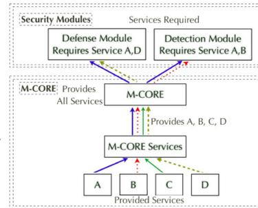
To implement a defense mechanism against Sybil Attacks, our *sybil* module uses the *rssivalue* interface (service) provided by the RSSI sub-module of the M-Core.
