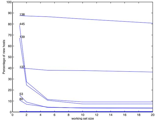
**Figure 8. Graph showing percentage of new hosts against working set size for traffic on different protocols. Each line is labelled except the three at the bottom which are 143, 8088, and 11000. All of the protocols exhibit some form of locality (number of new hosts reducing with working set size) except 137 and 138.**
