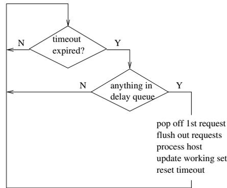
**Figure 2. Processing loop for rate limiting.** Whenever the timeout expires, if there is anything in the delay queue, the first request on that queue is processed. This involves flushing out any other requests to the same destination from the queue, making the connections, updating the working set with the new destination, and resetting the timeout.
