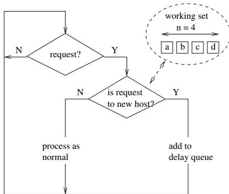
**Figure 1. Processing loop for new requests.** Whenever a request is made it is compared against a list of recently used hosts (shown in the dotted ellipse) to determine whether it is new or not. If the connection is to a new host, (e.g. to host ‘e’ which is not in the working set) it is placed on a delay queue to await processing, while if it is not new (say to host ‘b’), it is processed immediately.
