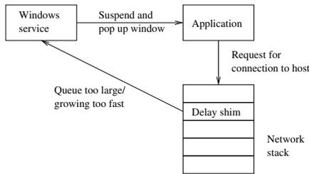
**Figure 9. A possible implementation of this system on the Windows platform based on the architecture of a software firewall. The delay queue and working set is implemented as a “shim” in the network stack. The queue becoming too large suggests the presence of an infected application, and a windows service is used to suspend the application and pop up a window asking the user for directions.**
