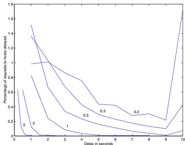
**Figure 7. Plot of simulation of filter, showing the proportion of requests that were delayed (as a percentage of the total number of requests) plotted against the time that they were delayed (in seconds). The different lines correspond to different values of  $r_{allowed}$ . This data is for user 1, with a working set size of 5. The delays are small and few requests are affected, particularly for higher values of  $r_{allowed}$  ( $< 1\%$  for  $1 < r_{allowed} < 5$ ).**
