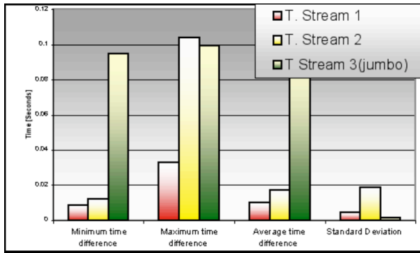
Figure 9: Minimum (leftmost), maximum (second leftmost), and average (third leftmost) packets interarrival time with std. deviation (rightmost) for three traffic streams (T. Stream 1: leftmost bar in each group, T. Stream 2: central bar in each group, T. Stream 3: rightmost bar in each group) with (T. Stream 1) and without QoS (T. Stream 2 and 3).
